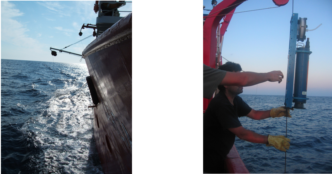
Figure 2.7: Tow-fish used during the Thresholds cruise for avoiding potential contamination of samples from the ship (left picture) and in-situ pump for sampling water at the deep chlorophyll maximum.
